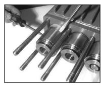
Remove the seal sleeve (35) from the manifold and /or crankcase.
