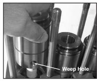
13) Replace complete seal sleeve (35)/seal case (37) assembly into crankcase (1). Make sure that the weep hole points downward. Note: To replace the oil seals (31), you will need to disassemble the gear end (see instructions below).
