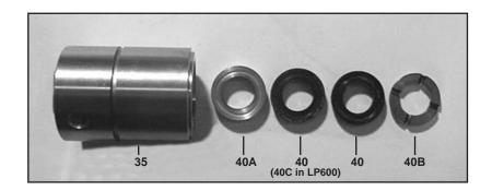
11) Remove the pressure ring (40A), v-sleeves (40), sleeve (40C in LP600 only), and support ring (40B), from the seal sleeve. For LP301A and LP301A-4000 pumps, remove the pressure spring (41). Examine seals carefully and replace if worn. Clean surfaces of seal sleeves (35) which come in contact with the crankcase (1) and sealing surfaces of valve casing (43).
