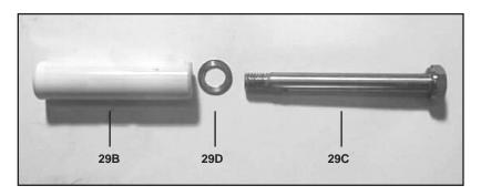
12) Check plunger surface (29B). If plunger pipe is worn out, loosen tension screws (29C) with a 15mm socket and pull off plunger pipe to the front. Clean front surface of plunger (29B) thoroughly. Apply a small drop of locktite to tension screw. Put a **new** crush washer (29D) onto tension screw. Put a thin coat of glue (Loctite) on the ring (or ceramic plunger side) and tighten screw to 265 in.-lbs. (30 NM).
